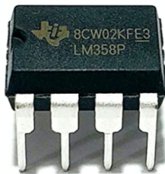
Figure 5: LM358 Low Power, Dual-Operational Amplifier
